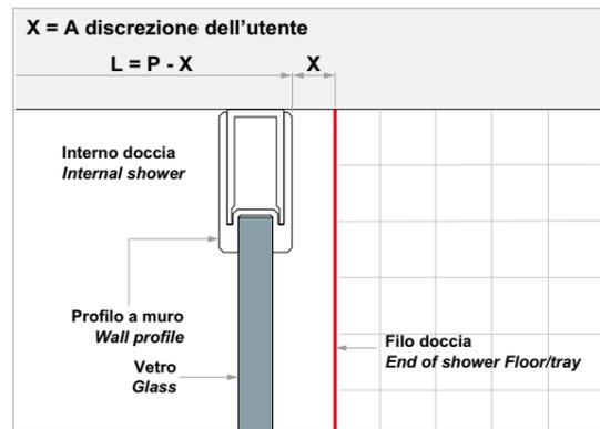
**MONTAGGIO SOPRA MEZZARIA VETRO** *Assembly on top of glass*
