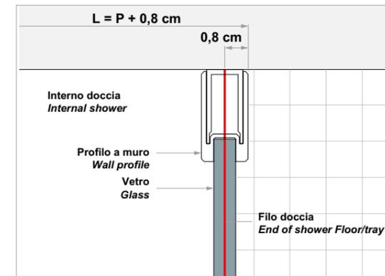
**MONTAGGIO VETRO INTERNO** *Assembly internal glass*
