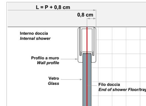
**MONTAGGIO VETRO INTERNO** *Assembly internal glass*
