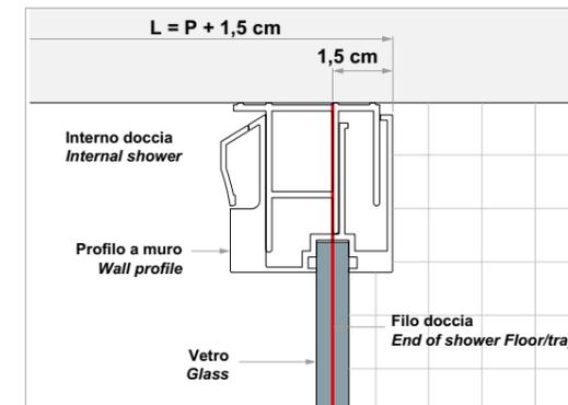
**MONTAGGIO VETRO INTERNO** *Assembly internal glass*
