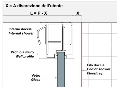
**MONTAGGIO SOPRA MEZZARIA VETRO** *Assembly on top of glass*
