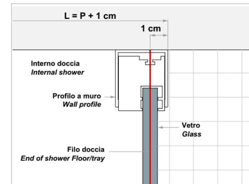
**MONTAGGIO VETRO INTERNO** *Assembly internal glass*
