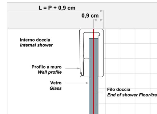
**MONTAGGIO VETRO INTERNO** *Assembly internal glass*
