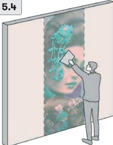
then, level the fiber glass roll with a plastic spatula avoiding any damage to the wallpaper face surface. In case there is not enough glue to perfectly apply the wallpaper rolls to the wall, add further glue on the face surface until the roll is completely covered.
