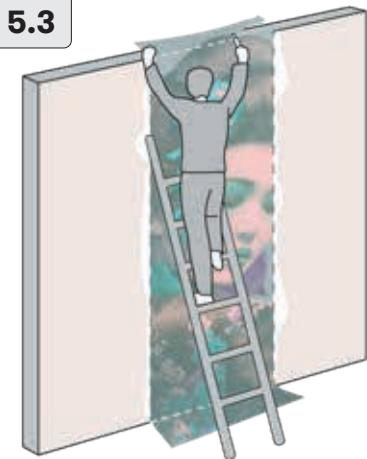
Cut the exceeding material on the ceiling and floor with a sharp cutter.
