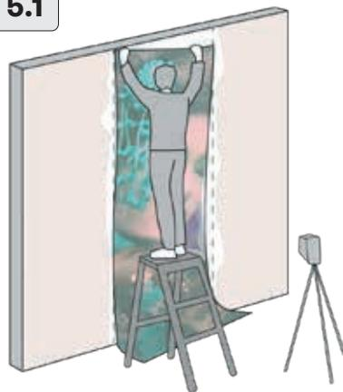
Apply the roll perpendicularly to the ground with the help of the laser level, taking care to leave an exceedance on both ceiling and floor side for about 5 cm.
